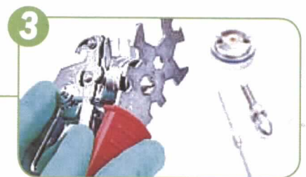
3 And finally, unscrew fluid tip with the ring spanner integrated in the universal wrench
